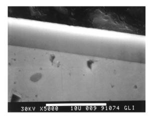
Figure 4. SEM image of the interfacial region at an IBED chromium coated copper surface. (SEM: AMR, Model 1000).
