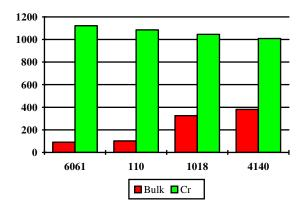
Figure 7. Knoop hardness measurements of the bulk material and the IBED chromium coating on each base material. The loading force used for these measurements was 5 grams.
