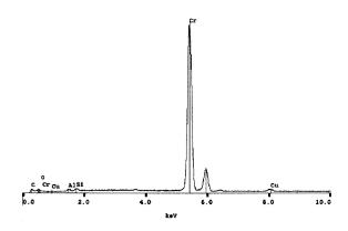
Figure 5. X-ray photoelectron spectrum from the IBED chromium layer. (Princeton GammaTech - IMIX Spectrometer).
