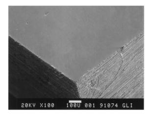
Figure 3. SEM image of a 5 micron (0.0002 inch) thick coating of pure chromium on a polished copper substrate. (SEM: AMR, Model 1000).
