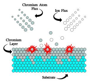
Figure 2. Schematic diagram of the implementation of the IBED process. Growth of a pure chromium coating is shown. Other metallic coatings, such as titanium, aluminum, copper, silver, and gold can also be deposited with the IBED process.
