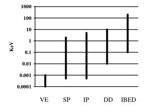
Figure 1. The arrival energy ranges of coating particles found with the five general classes of coating deposition processes.
