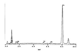
Figure 6. X-ray photoelectron spectrum from the copper substrate. (Princeton GammaTech - IMIX Spectrometer).
