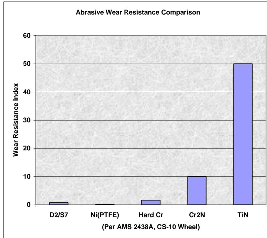
**Figure 1: Comparative Wear Resistance of Various Coatings**
