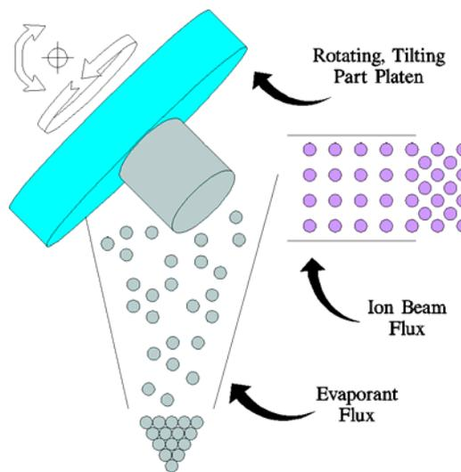
Figure 4. Punches and dies are mounted to a rotating, tilting part platen that allows the coatings to be deposited uniformly on all tooling surfaces, including all embossed features.
