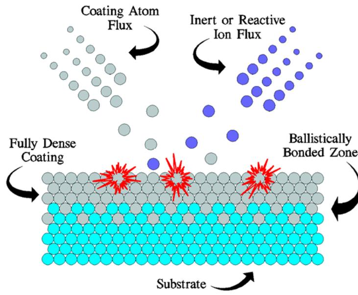
Figure 3. IBED coatings are deposited by vapor depositing a coating on the punch surface and augmenting the coating adhesion and growth with an energetic ion beam. Processing is done in a vacuum chamber at temperatures that do not exceed 150 degrees Fahrenheit.
