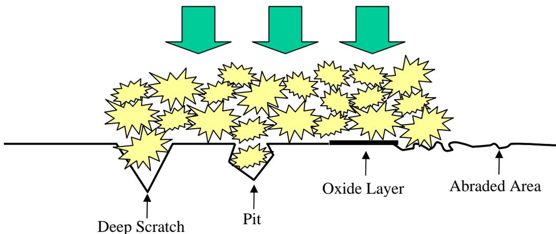
Figure 2. Powders compressed against a roughened surface can become trapped in scratches and pits causing powder build-up, eventually leading to sticking and picking.
