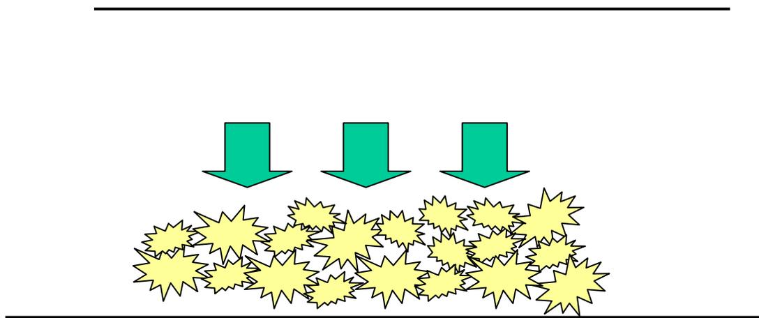
Figure 1. Powders compressed against a smooth polished surface show no mechanical interlocking with the surface and sticking and picking are minimized.
